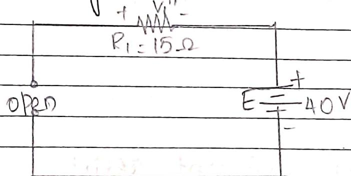
By applying Ohm's law, can calculate voltage ( $V_1''$ ) for ' $E$ ' and ' $R_1$ '.
